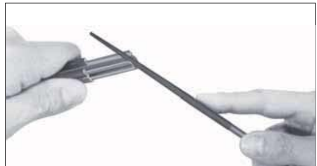
Photo 9: Remove inside burr with round file
